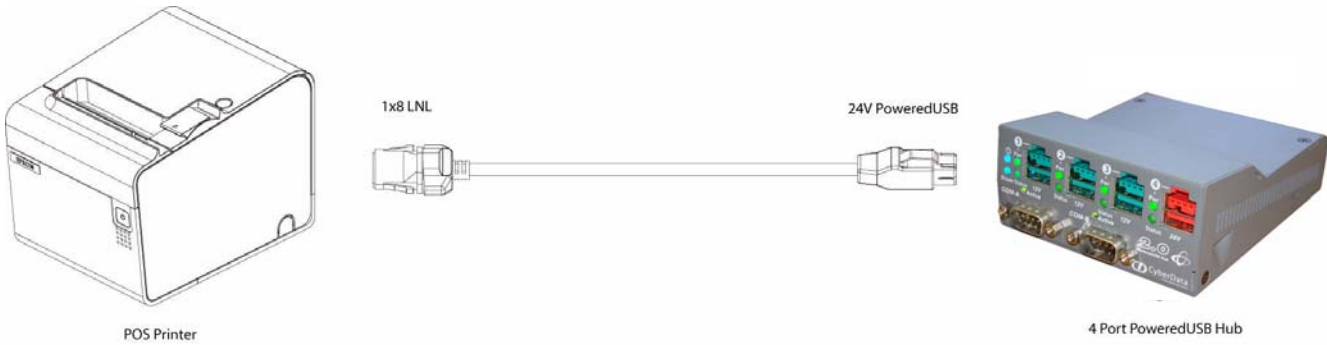
Figure 2-13. Cable, +24V PoweredUSB to 1x8 PoweredUSB
