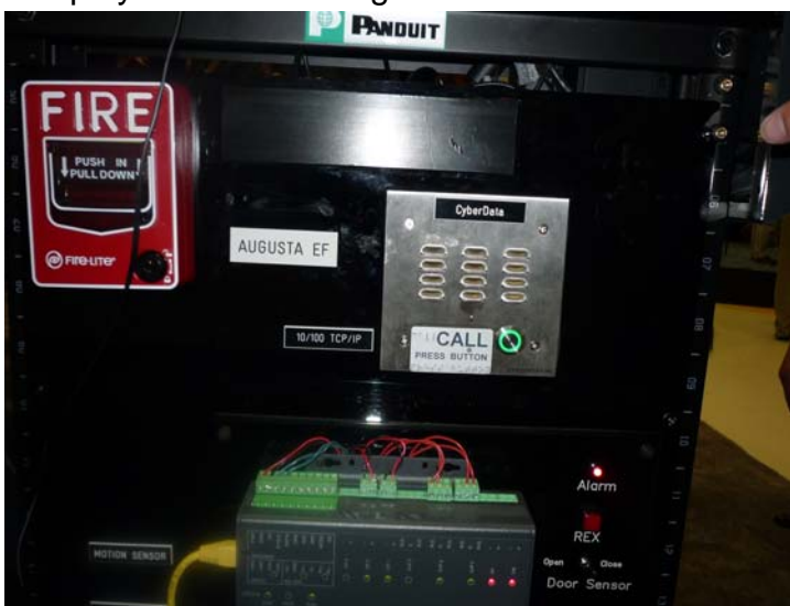
Figure 2 CyberData's VoIP Intercom on display as part of Cisco's Open Platform for Safety & Security Solutions.
